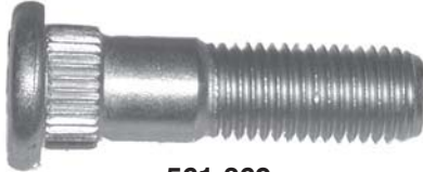
561-369 M12 x 1.5 x 46mm Knurl diameter: 15mm
