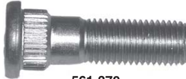
561-370 M12 x 1.5 x 44mm Knurl diameter: 15.8mm
