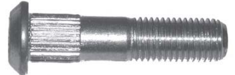
561-255 M12 x 1.5 x 52mm Knurl diameter: 12.9mm (Code M.Z.2)
