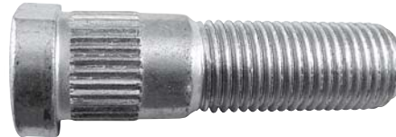
561-502 M14 x 1.5 x 50mm Knurl diameter: 16.02mm
