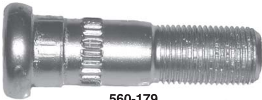
560-179 5/8-18R x 2-3/8" Knurl diameter: .720 (Code: GF)
