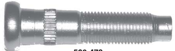
560-473 9/16-18R x 2-5/8" Knurl diameter: .622 (Code:CX)
