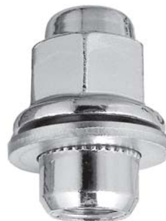
559-117 M12R x 1.5 21mm Hex 37mm Height 18.4 dia. flg. x 11.9 lg. Chrome
