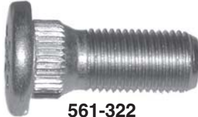
561-322 M12 x 1.25 x 30.2mm Knurl diameter: 14.27mm
