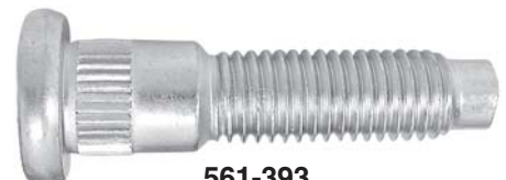
561-393 M12 x 1.75 x 55mm Knurl diameter: 14.6mm
