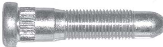
561-428 M14 x 1.5 x 65mm Knurl diameter: 15.7mm
