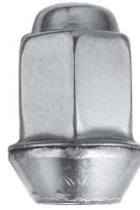
558-071 1/2-20R 13/16" Hex 1-15/32" Height Stainless Steel Capped
