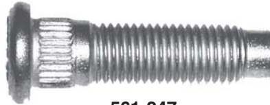
561-247 M12 x 1.5 x 46mm Knurl diameter: 13.41mm
