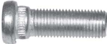
561-413 M14 x 1.5 x 43mm Knurl diameter: 15.7mm (Code PU)
