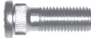
561-140 M12 x 1.5 x 37mm Knurl diameter: 14.4mm (Code M.1.8)
