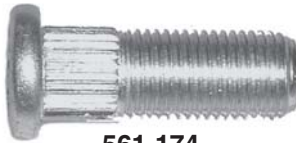
561-174 M12 X 1.25 x 34mm Knurl diameter: 12.24mm (Code: BA)
