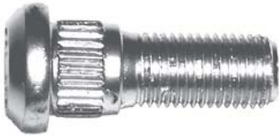
560-386 7/16-20R x 1-5/16" Knurl diameter: .555 (Code: DN)
