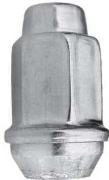
558-094 1/2-20R 3/4" Hex 1-39/64" Height Stainless Steel Capped
