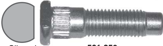
561-250 M12 x 1.5 x 47mm Knurl diameter: 13.34mm
