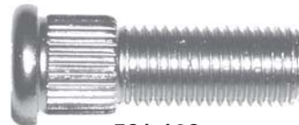
561-106 M12 x 1.5 x 38.5mm Knurl diameter: 14.7mm (Code M.2.0)
