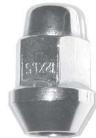
559-077 M12 x 1.5 Acorn Bulge 19mm (3/4") Hex 35mm Height Cone Angle: 60° Chrome
