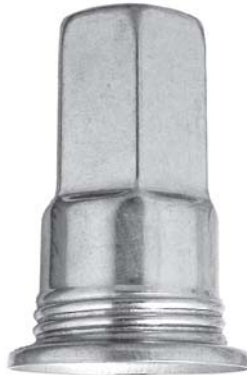
559-201 M24 x 2.0 Thread 19mm Hex Stainless Steel
