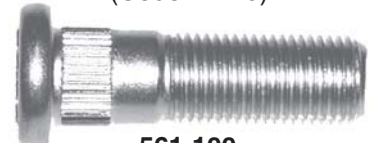
561-100 M12 x 1.25 x 39mm Knurl diameter: .12.9mm (Code: D.1.0)
