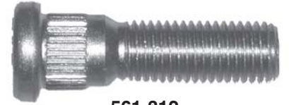
561-312 M12 x 1.5 x 44.4mm Knurl diameter: 14.17mm
