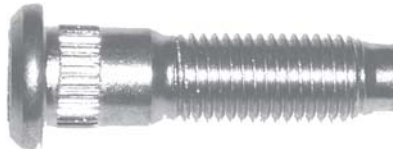
561-251 M12 x 1.5 x 51mm Knurl diameter: 13.5mm (Code F.1.1)
