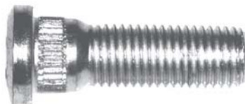
561-126 M12 x 1.5 x 41mm Knurl diameter: 14.2mm (Code T.6.0)
