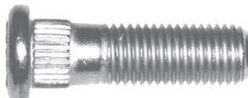
561-169 M12 x 1.5 x 43mm Knurl diameter: 12.85mm (Code Cl)
