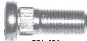
561-401 M12 X 1.25 x 42mm Knurl diameter: 14.43mm
