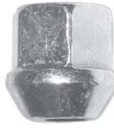
559-163 M12 x 1.5 19mm (3/4") Hex 23mm Height Cone Angle: 60° - Zinc
