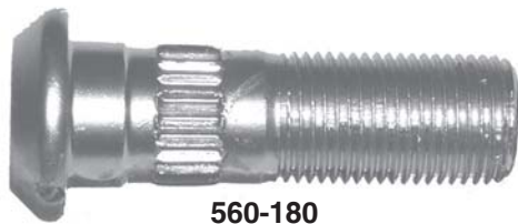
560-180 5/8-18R x 2-1/16" Knurl diameter: .655 (Code: GI)
