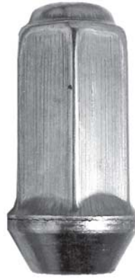
558-143 1/2-20R 13/16" Hex 2-1/32" Height Stainless Steel Capped
