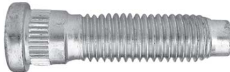
561-442 M14 x 2.0 x 58mm Knurl diameter: 15.5mm
