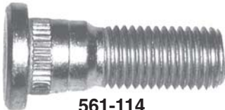
561-114 M12 x 1.5 x 38mm Knurl diameter: 14.35mm (Code C.U.1)
