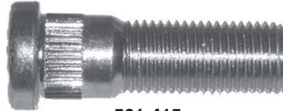
561-415 M14 x 1.5 x 46mm Knurl diameter: 15.8mm (Code DO)
