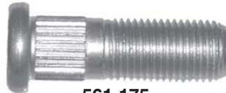
561-175 M12 x 1.25 x 38mm Knurl diameter: .12.24mm (Code: BC)
