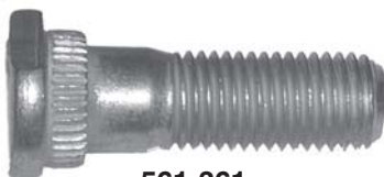
561-361 M12 x 1.5 x 41.0mm Knurl diameter: 16.5mm
