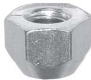
559-172 M12 x 1.5 21mm (13/16") Hex 18mm Height Cone Angle: 60° - Zinc
