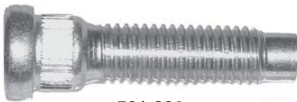
561-390 M12 x 1.75 x 51mm Knurl diameter: 14.73mm
